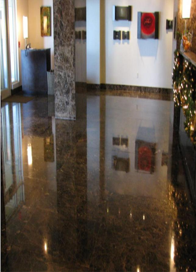
The crystallization process consists of spraying a liquid onto the marble floor and buffing it in with steel wool under a standard speed floor machine. The steel wool generates heat through abrasion and the chemical reacts with the marble, producing a new compound on the surface of the stone.
